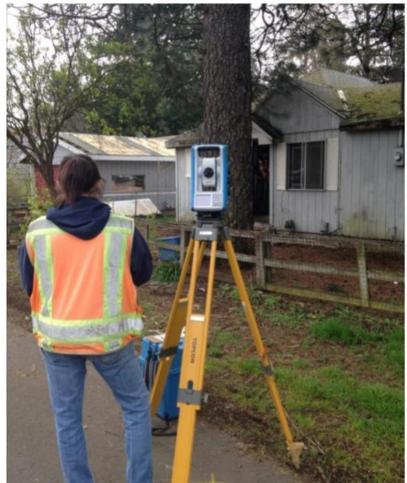
*Surveyor taking measurements for an elevation certificate.*
